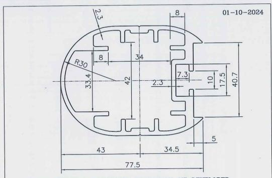
AS PER CUSTOMER REFERENCE DIMENSIONS WE DEVELOPED THIS DRAWING BUT WE FOUND SOME ERROR IN DRAWING. PLEASE CHECK ALL DIMENSIONS AND MATCH WITH MATCHING PART.
