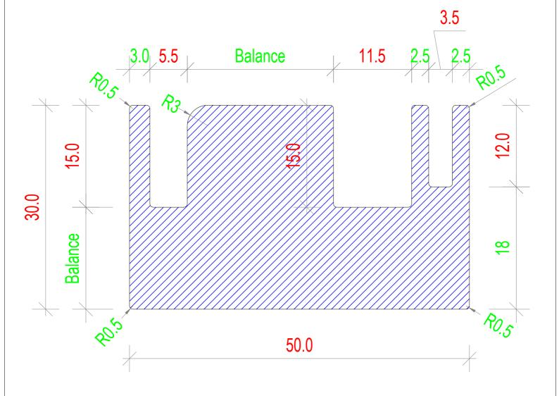
CRITICAL DIMENSIONS ARE MARKED IN 'RED' ALL DIMENSIONS ARE IN MM, TOLERANCE =  $\pm 0.2$ MM
