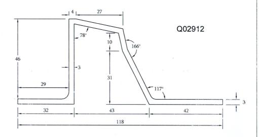
C. S. Area = 579.10 mm Sq.Weight Per Meter Length =  $2.72 \times 603.58 \times 10^{-3} \times 10^{-3} \times 1000$ = 1.57 Kg / Meter
