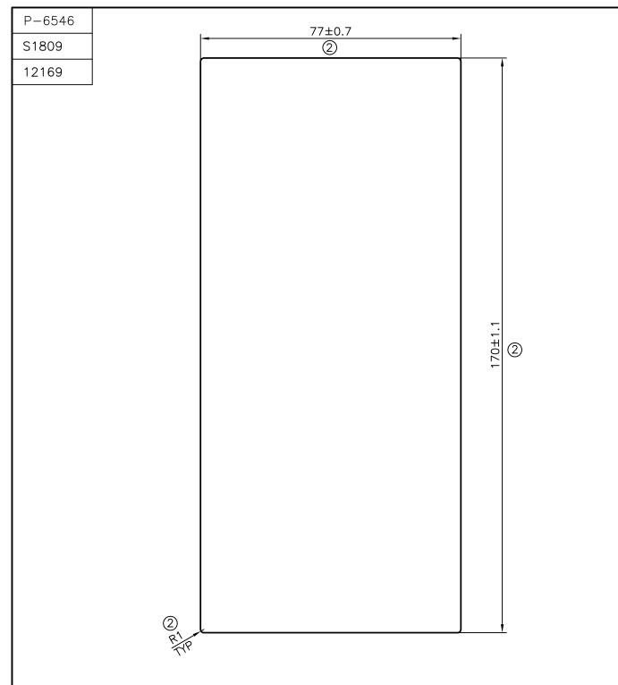
ISSUE- ② DIMENSIONS CHANGED FROM 75.0 mm TO 77.0 mm, 168.0 mm TO 170.0 mm & WEIGHT ALSO CHANGED FROM 34.018 kg/m TO 35.341 kg/m
