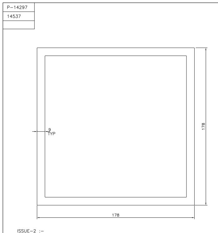
SIZE CHANGED FROM 180 TO 178 mm & THICKNESS CHANGED 10 mm TO 9mm
