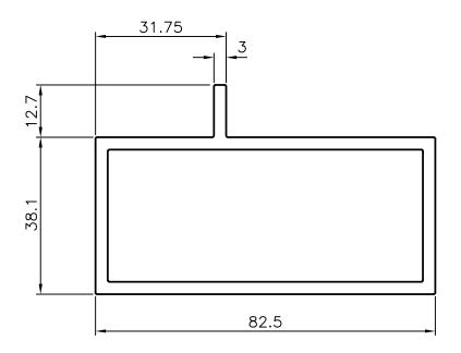
TYPICAL WALL THICKNESS :- 3mm
