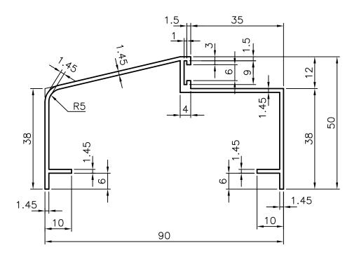
1.TOLERANCES ON DIMENSIONS, STRAIGHTNESS, FLATNESS, TWIST AND ANGULARITY WILL BE AS PER IS: 3965-1981
