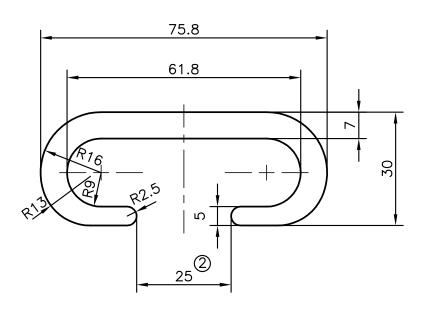
ISSUE-2 DIMENSIONS CHANGED FROM 27.8 mm TO 25 mm WEIGHT ALSO CHANGED FROM 2.431 kg/M TO 2.469 kg/M  $\,$
