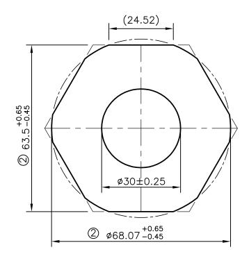
ISSUE - ② TOLERANCE CHANGED FROM  $68.07\pm0.45$  TO  $\phi68.07^{+0.65}_{-0.45}$  AND  $63.5\pm0.45$  TO  $63.5^{+0.65}_{-0.45}$  AND OUTER SHAPE ALSO CHANGED AS PER CUSTOMER REQUIRMENT
