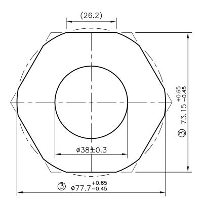
ISSUE - ③ TOLERANCE CHANGED FROM 77.7 $\pm$ 0.45 TO  $\phi$ 77.7 $\pm$ 0.45 AND 73.15 $\pm$ 0.45 TO 73.15 $\pm$ 0.45 AND OUTER SHAPE ALSO CHANGED AS PER CUSTOMER REQUIRMENT
