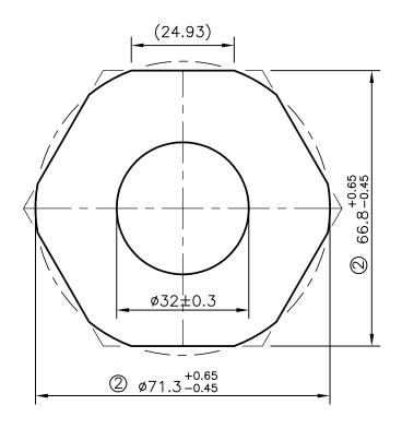
ISSUE - ② TOLERANCE CHANGED FROM 71.3 $\pm$ 0.45 TO Ø71.3 $^{+0.65}_{-0.45}$  AND 66.8 $\pm$ 0.45 TO 66.8 $^{+0.65}_{-0.45}$  AND OUTER SHAPE ALSO CHANGED AS PER CUSTOMER REQUIRMENT
