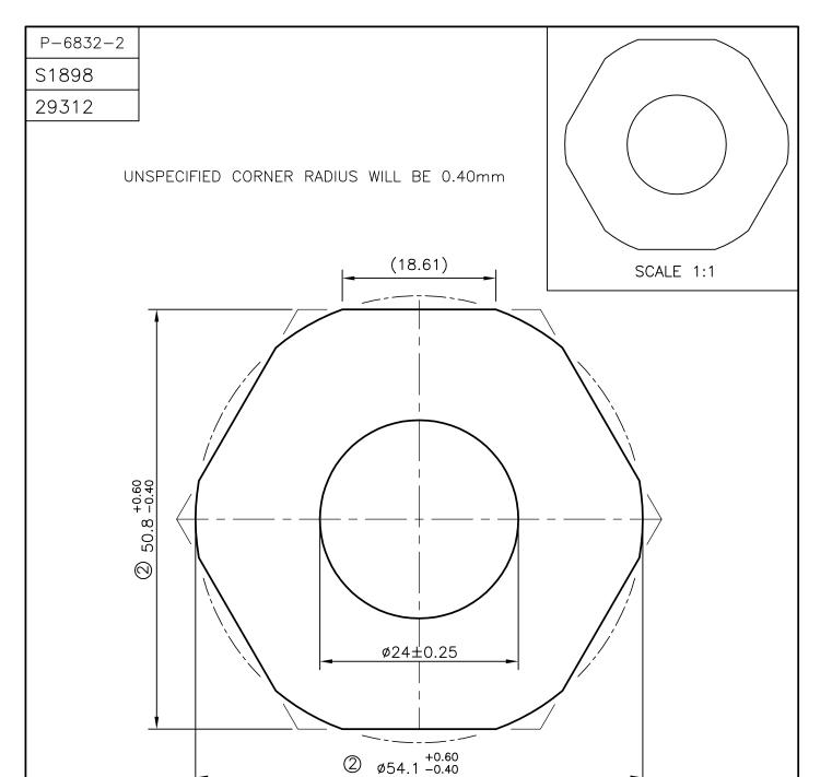
ISSUE - ② TOLERANCE CHANGED FROM 54.1 $\pm$ 0.4 TO  $\phi$ 54.1 $^{+0.60}_{-0.40}$  AND 50.8 $\pm$ 0.4 TO 50.8 $^{+0.60}_{-0.40}$  AND OUTER SHAPE ALSO CHANGED AS PER CUSTOMER REQUIRMENT
