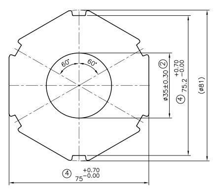
ISSUE-2 :- I.D. CHANGED FROM Ø 38 TO Ø35 mm WEIGHT ALSO CHANGED FROM 9.511 TO 9.976 kg/M ON DATED 20/07/2009
