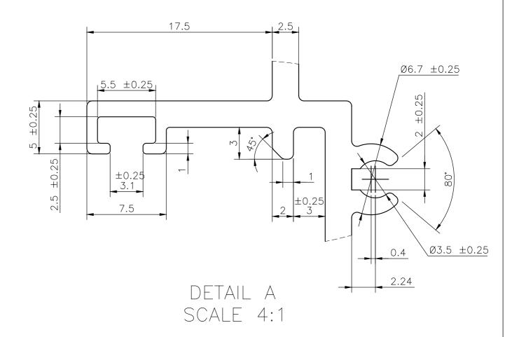
$TWIST = \pm 1/4^{\circ}/300M.M./M.$  FLATNESS = WIDTHX0.005mm. STRAIGHTNESS = 1.5 M.M./MTR.
