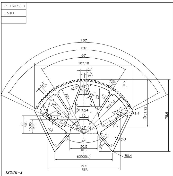
\* MARKED RADIUS CHANGED FROM 1.0 TO 3.0 mm DIMENSIONS CHANGED FROM 20 TO 18.24 & 53 TO 51.92 WEIGHT ALSO CHANGED FROM 4.992 kg/m TO 5.159 kg/m
