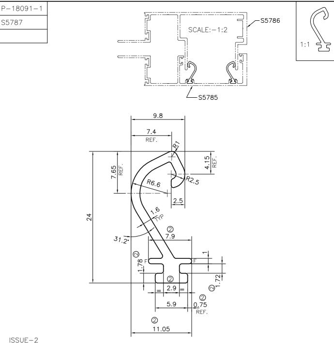
DIMENSION CHANGED FROM 10.3 mm TO 11.05 mm & FROM 5.4 TO 7.9, FROM 2.5 TO 2.9 DIMENSION CHANGED FROM 0.25 REF. TO 0.75 REF. mm & FROM 1.75 TO 1.72 mm THICKNESS CHANGED FROM 1.75 TO 1.78 mm
