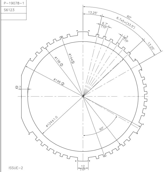
DIMENSION CHANGED FROM Ø140 mm TO Ø144 mm, Ø134 mm TO Ø138 mm, DIMENSION CHANGED FROM Ø142 mm TO Ø146 mm & Ø123 mm TO Ø124 mm, THICKNESS CHANGED FROM 5.5 TO 7.0 mm
